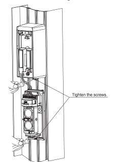
8 After completing the settings and operation check, insert the tamper bushing into each transmitter/receiver.
