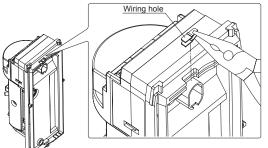
5 Remove the chassis from the back box.
