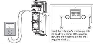
5 Set the voltmeter range to 5 to 10 VDC. After checking the receiving level of optical axis by using the alarm indicator, make sure to make fine alignment for both transmitter and receiver with voltmeter until it reaches maximum monitor output over "good" level.
