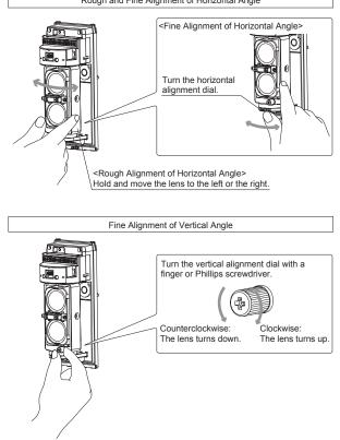
3 Adjust the horizontal and vertical angles while checking the light receiving status by Alarm indicator LED on the pairing receiver.
