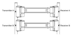
Since Receiver B may receive the infrared beam from Transmitter A, select the frequencies as shown in the figure above. (In the figure, each number in the square indicate a channel numbers.)
