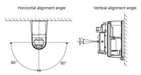
Optical alignment is an important adjustment to increase reliability. Be sure to take adjustment steps 1 through 5 described below to attain the maximum level of the output through the monitor jack.
