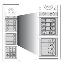
In manual programming the call keys are arranged as in the diagram for a maximum of 98 keys.
