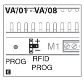
When programming is completed, place the RFID PROG jumper as shown in figure  $\blacksquare$ .
