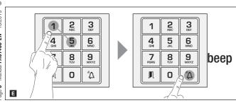
Press the door-release — and AUX2 keys and enter the group call code (from 1 to 98) followed by key  $\triangle$ : The call code is associated with the internal receiver  $\square$  and the call key chosen  $\square$ . Continue, repeating the same operations for all the other internal receivers. The operation can only be carried out from an entry panel with the  $\not \triangle$  LED off.
