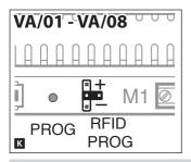
When programming is completed, place the RFID PROG jumper as shown in figure  ${\bf K}$ .
