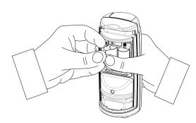
Figure 16: Pulling the battery tab
