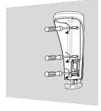
Figure 6: Fastening the bracket
