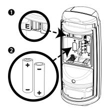
Figure 15: Enrollment button and battery polarity
