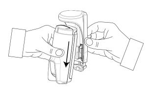
Figure 13: Removing the detector from bracket
