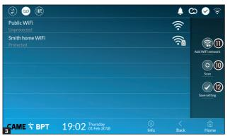
The page shows the detected networks; to manually scan for networks, touch the **10** button.
