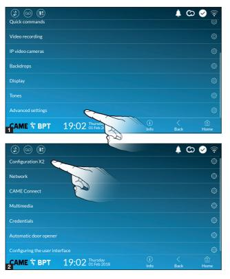
This section requires specific know-how in operating the video-intercom system. Wrong settings may cause partial or even total malfunctions; that is why the editing of some parameters is allowed only after entering the installer password; the default password is 112233).
