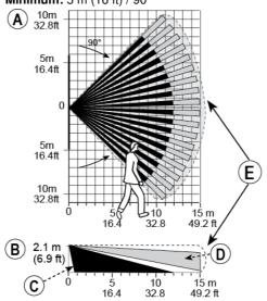
Figure 5. Coverage Pattern & Walk-test
