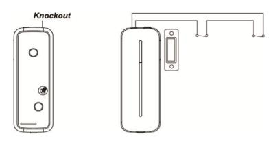
• The extension terminal and internal magnetic switch can function together to trigger the Door Contact when either of them is activated, you can also choose to disable the internal magnetic switch through JP3 Jumper setting. If both extension terminal and internal magnetic switch is in use and any of them is triggered (opened). The Door Contact will only send Door Contact close (restore) signal when both of them are closed.
