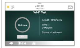
A successful test will result in a "pass" and indicates the date and time of the test along with connection speed. To perform a Wi-Fi Test, touch the "Run" button.
