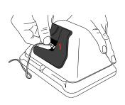
1. Locate the IQ Base with SmartMount and connect the power cable from the IQ Base into the **BLACK** connector inside the IQ Panel 4. Refer to Interior Diagram on Page 7
